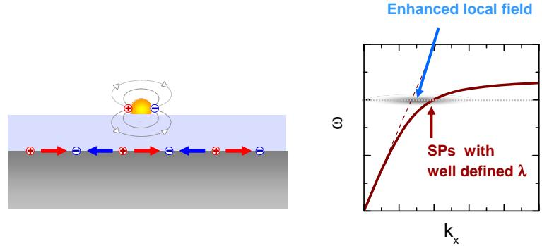
The diagram shows a yellow circular nanostructure on a grey substrate, representing resonance. The plot shows the dielectric function  $\epsilon$  on the y-axis and wave vector  $k_x$  on the x-axis. A red curve represents 'SPs with well defined  $\lambda$ ', while a dashed line represents 'Enhanced local field'. A blue arrow points to the dashed line.
