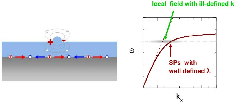
The diagram shows a blue circular nanostructure on a grey substrate. A dipole moment is indicated by a red '+' and a blue '-' with arrows. The plot shows the dielectric function  $\epsilon$  on the y-axis and wave vector  $k_x$  on the x-axis. A red curve represents 'SPs with well defined  $\lambda$ ', while a dashed line represents 'local field with ill-defined  $k$ '. A green arrow points to the dashed line.
