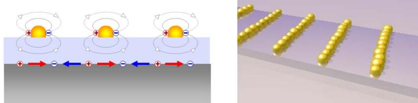
**Prediction:** surface plasmon excitation using resonant metal particles can be used to construct **miniature couplers**
