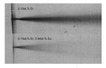
FIG. 6. False color image of the green emission of  $\text{Er}^{3+}$  with and without europium. The green emission from the  $\text{Er}^{3+} {}^{4}S_{3/2}$  state is represented in black. 980 nm light is coupled into the planar waveguide from a fiber (left hand side of the images). In the presence of 0.44 at. % europium, the green upconversion emission is reduced considerably.
