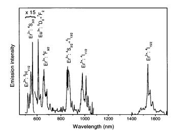
FIG. 2. Typical emission spectrum of an  ${\rm Er}^{3+}$  and  ${\rm Eu}^{3+}$  doped Y<sub>2</sub>O<sub>3</sub> waveguide, excited at 488 nm. Where no final state for a transition is given, the excitation relaxes directly to the ground state of the relevant ion.
