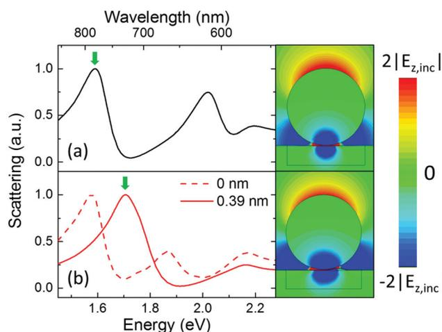
**Fig. 4** Normalized scattering spectra of a gold nanoparticle (a) on a 4-MBT coated flat gold film and (b) on a corrugated gold surface with  $d = 0$  (dashed line) and  $d = 0.39$  nm (solid line). The field-plots show two-dimensional electric field distributions at the main resonance peak of the spectra as indicated by the green arrows.
