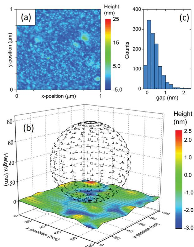
**Fig. 2** (a) AFM image of a gold film thermally evaporated on glass. (b) Example surface geometry near a liquid-deposited gold nanoparticle deposited on top of the surface shown in (a). (c) Normalized gap size histogram from over 1200 possible particle locations.
