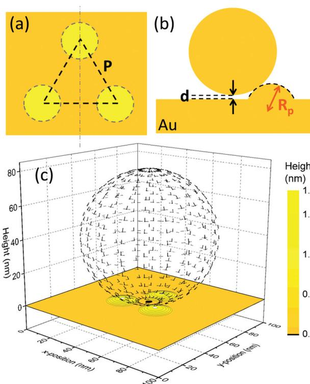
**Fig. 3** Schematic of a representative simulation geometry and relevant parameters showing (a) a top view without a gold nanoparticle showing three protrusions, (b) a side view along the dashed line in (a) with a deposited gold nanoparticle present, and (c) a perspective view of the final structure.
